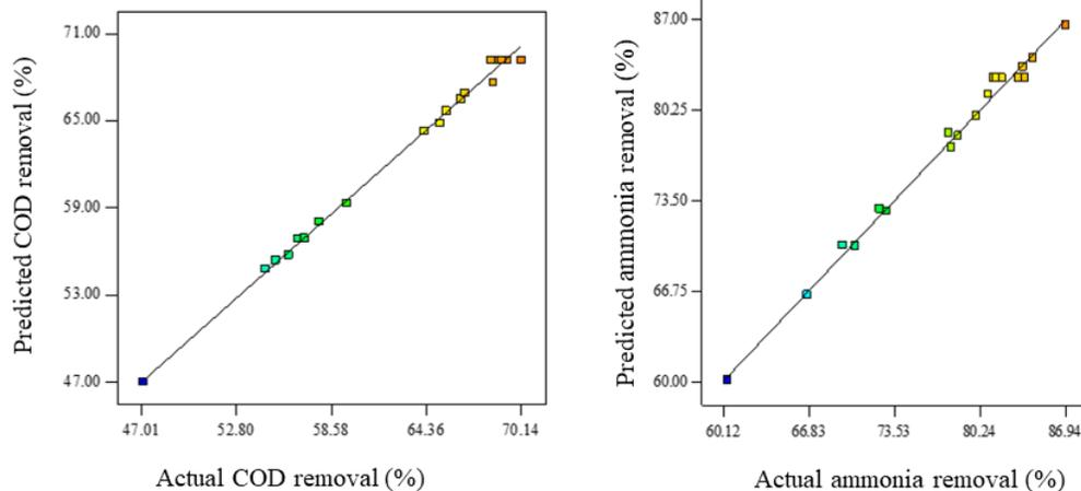
Fig.2 Predicted versus actual values plot for COD and NH<sub>3</sub>-N removal
