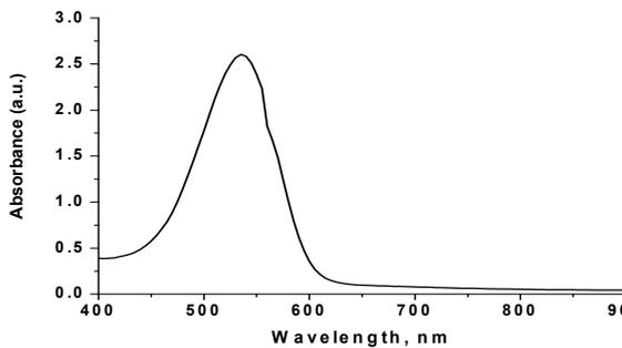
Fig. 6 : The dye absorption spectrum of dragon fruit dye in range of 400 nm to 900 nm.
