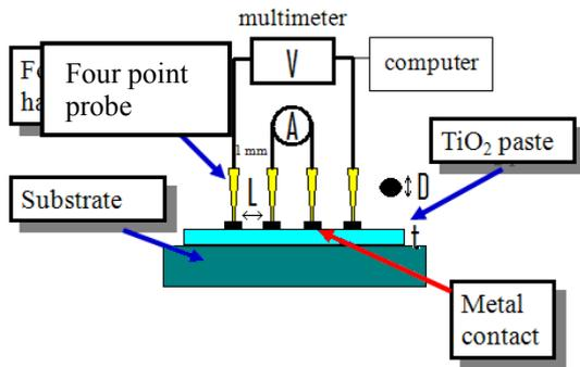
Fig. 4 : Computerized four hand probe diagram to characterize TiO<sub>2</sub> film with metal contact
