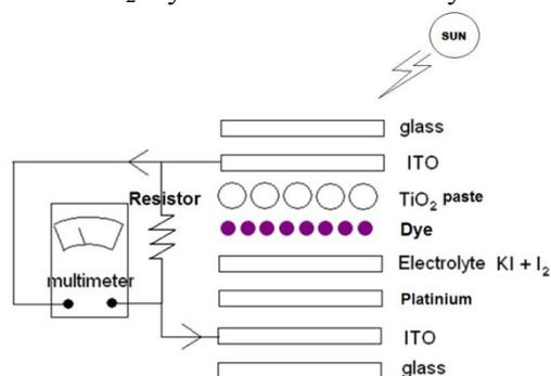
Fig. 1 The cross section assemble consist of ITO glass,  $\text{TiO}_2$  film, dragon fruit dye, electrolyte and platinum layer on ITO glass,
