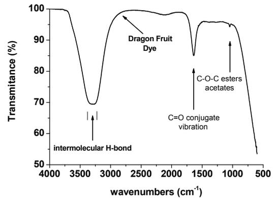
Fig. 7: The FTIR result of dragon fruit dye ranging from 4000  $\text{cm}^{-1}$  to 600  $\text{cm}^{-1}$ .
