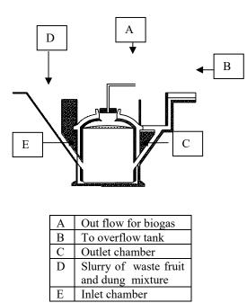
Figure 1 Schematic diagram of biogas digester
