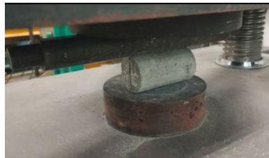
Fig. 7 SCC cylindrical specimen positioned for split tensile strength test
