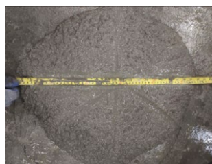
Fig. 3 Slump flow test
