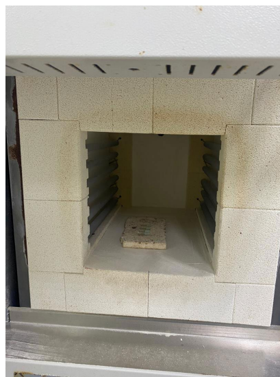
Fig. 2 \text{TiO}_2 coated substrate in the furnace to anneal
