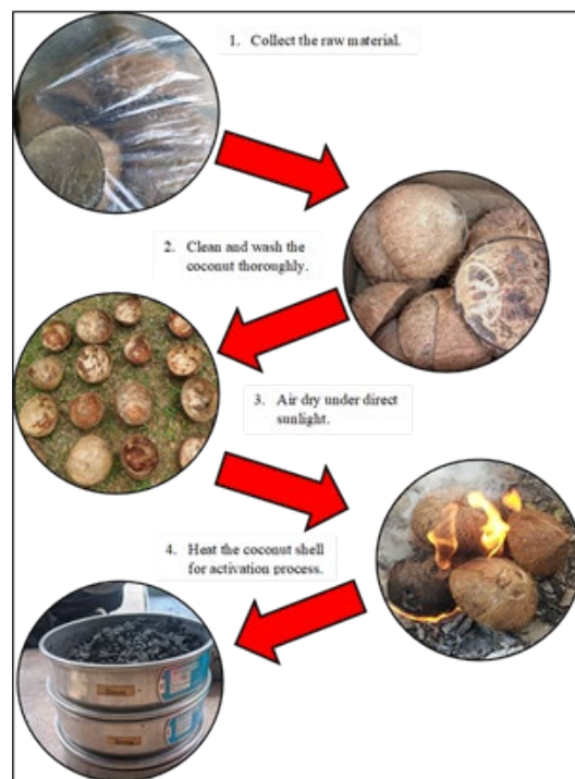
Fig. 3 Process flow for the production of burnt-crushed coconut shell
