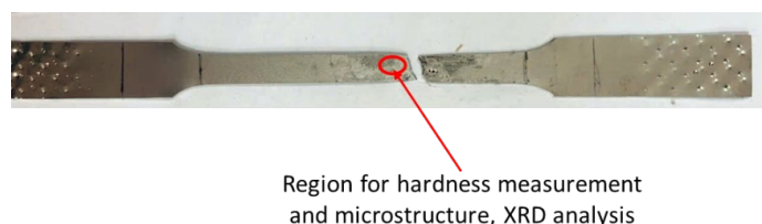
Fig. 10 Region for microstructure observation and XRD analysis after tensile test
