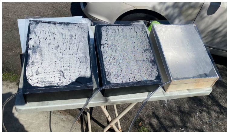
Fig. 3 Process of treating carwash wastewater using 3 different models of solar still distillation
