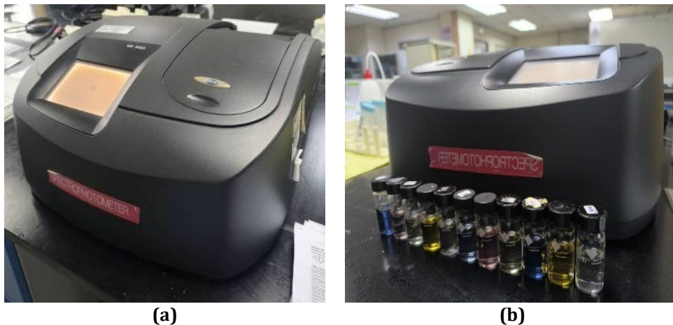
Fig. 3 (a) Spectrophotometer DR5000; and (b) Example of after analysing the samples
