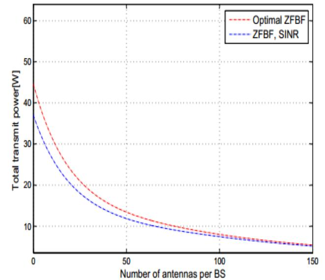
Fig. 4 Total transmit power versus number of antennas per BS.
