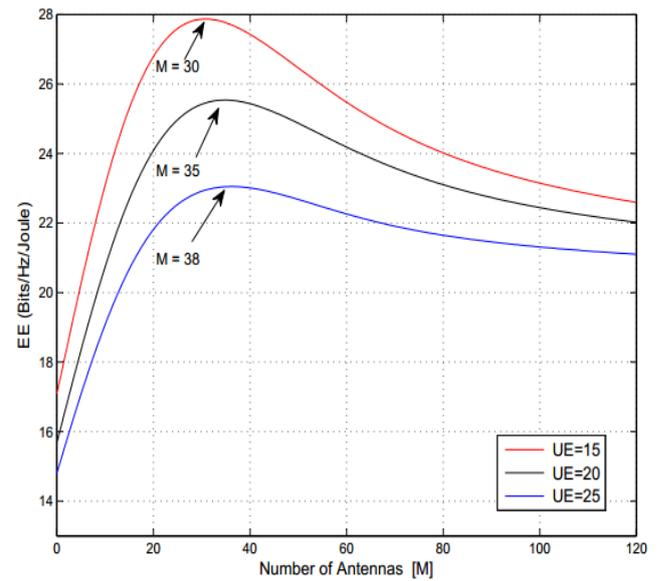
Fig. 3 Performance EE with the number of antennas  $M$ .
