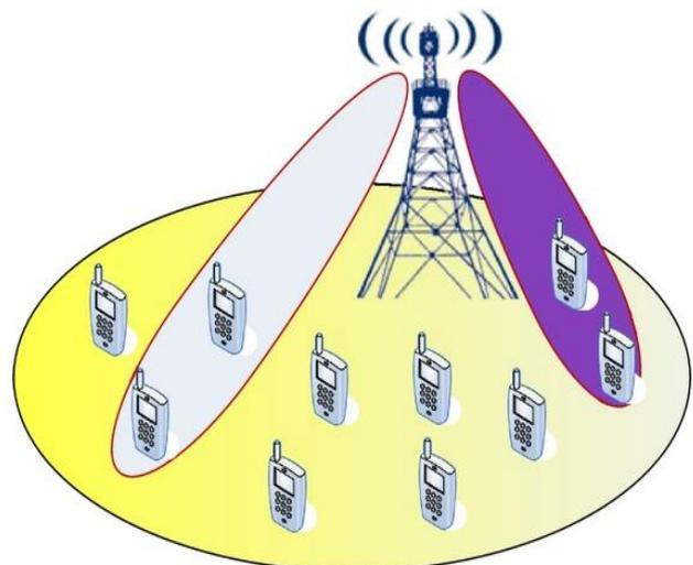
Fig. 1 Beamforming antennas in a single-cell massive MIMO system.
