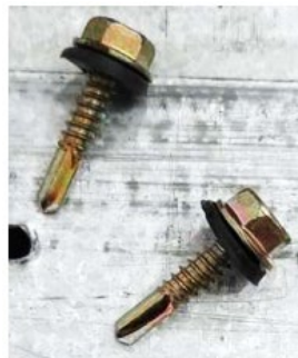
Fig. 3 Self-drilling screw as stud connector
