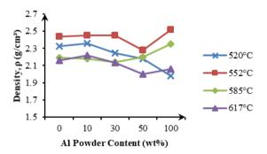
Fig. 4 Changes of density  $(g/cm^3)$  against sintering temperature of samples.
