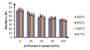
Fig. 6 The graph of hardness  $(H_V)$  against different sintering temperatures with increasing Al powder content.
