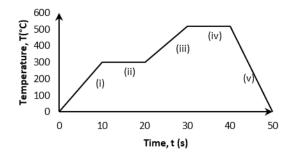
Fig. 1 Sintering profile.
