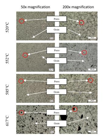
Fig. 3 The microstructure analysis of aluminium powder at four different sintering temperature
