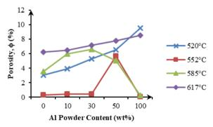
Fig. 5 The apparent porosity (%) against sintering temperatures with increasing Al powder content.
