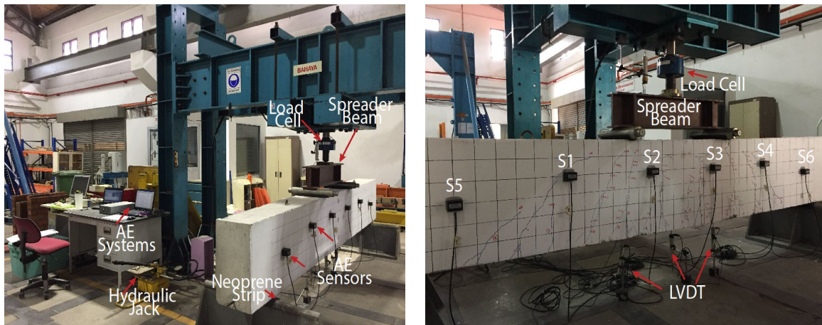
Fig. 5 Experimental setup for CLT and AE monitoring
