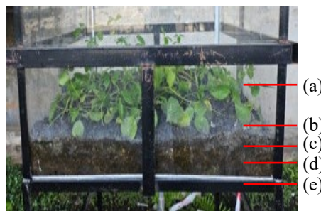
Fig. 2 Arrangement of green roof layers: (a) Vegetation; (b) Substrate; (c) Filter; (d) Drainage; and (e) Waterproofing
