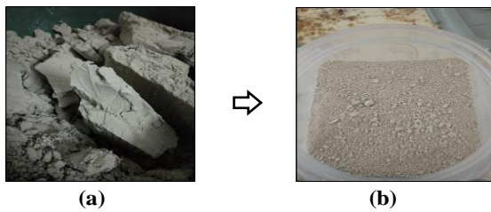
Fig. 1 Porcelain ceramic preparation: a) clay to b) powder
