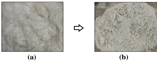
Fig. 2 AR glass preparation: a) fibre to b) milled powder
