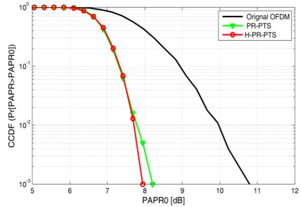
Fig. 3 Comparison between the H-PR-PTS and PR-PTS when  $N= 128$
