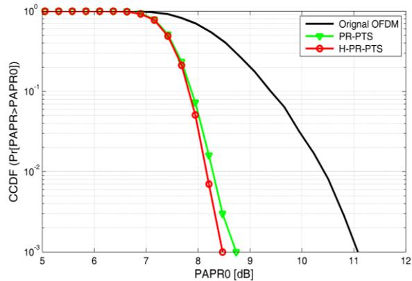
Fig. 4 Comparison between the H-PR-PTS and PR-PTS when  $N= 256$
