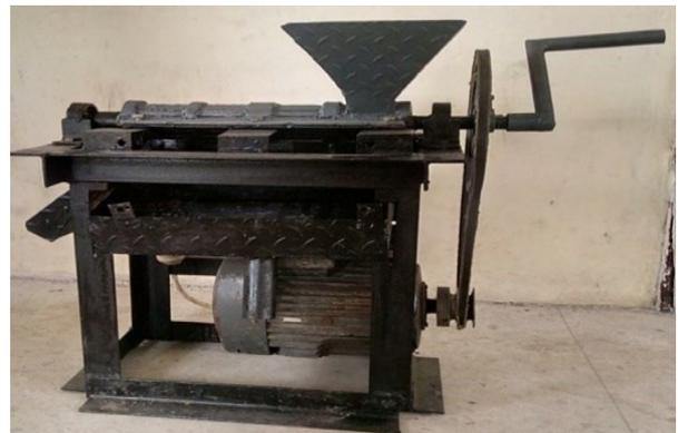
Fig. 2 Schematic set-up of palm kernel seed expeller.
