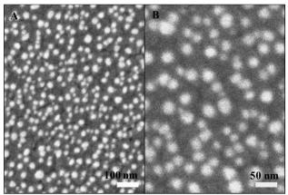
Fig. 7 FESEM image of gold nanosphericals obtained by grown using gold seed at magnification (a) 50K and (b) 100K.
