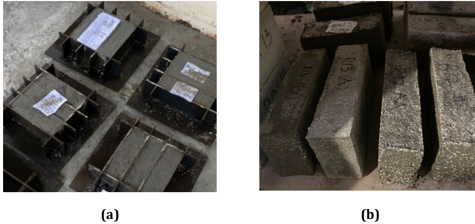
Fig. 3 (a) Cement sand brick casting; (b) Air curing
