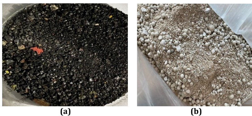
Fig. 1 (a) Copper slag; (b) Spent catalyst after grind
