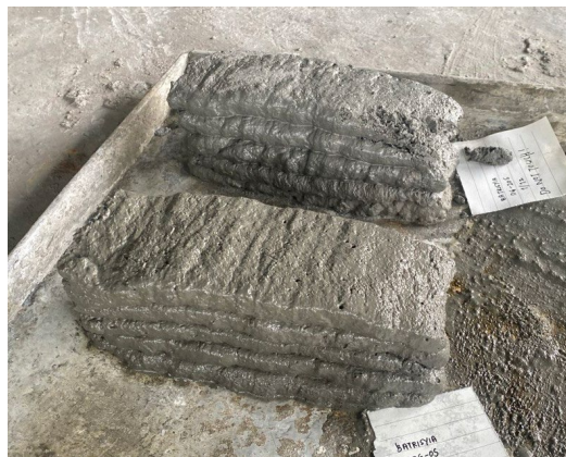
Fig. 3 Specimen of buildability test
