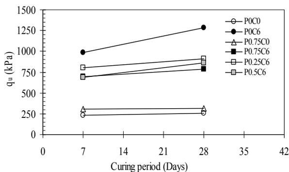
Fig. 5: Unconfined compressive strength – curing period.
