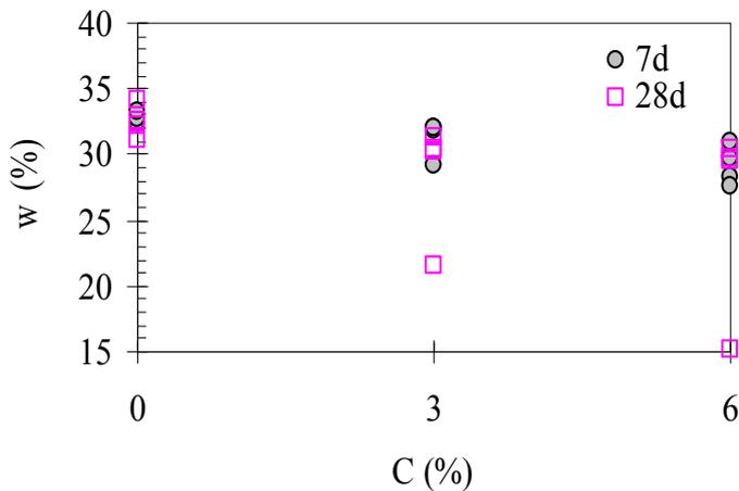
Fig. 2: Water content – cement content
