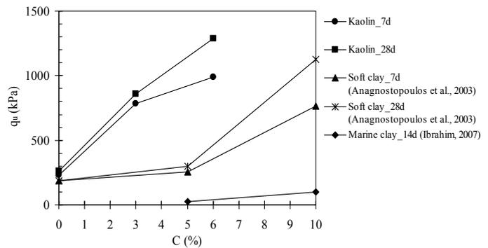
Fig. 6: Comparison of  $q_u$  for cement treated soils
