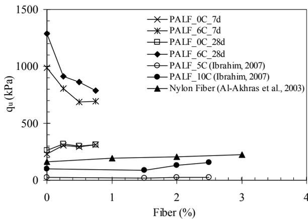
Fig. 7: Comparison of  $q_u$  for fibre-treated soils
