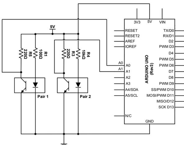
Fig. 4 Schematic diagram of the bee counter system
