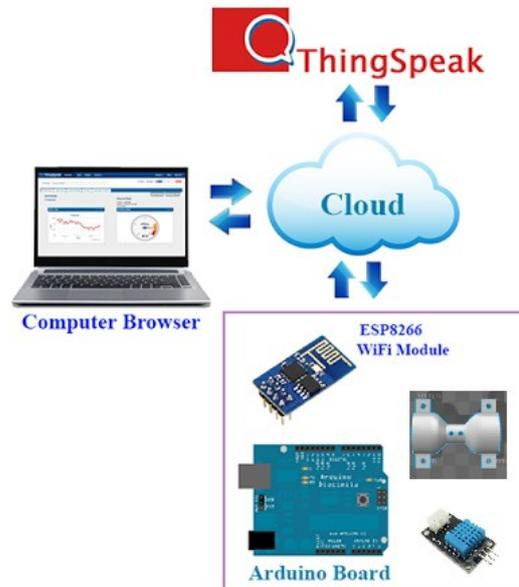
Fig. 6 Arduino and ESP8266 monitoring device with ThingSpeak
