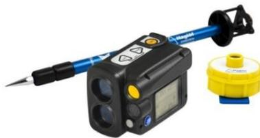
Fig. 11 Tree height laser instrument
