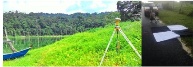
Fig. 7 Observation of GPS on GCP
