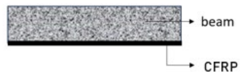
Fig. 3 CFRP plating design
