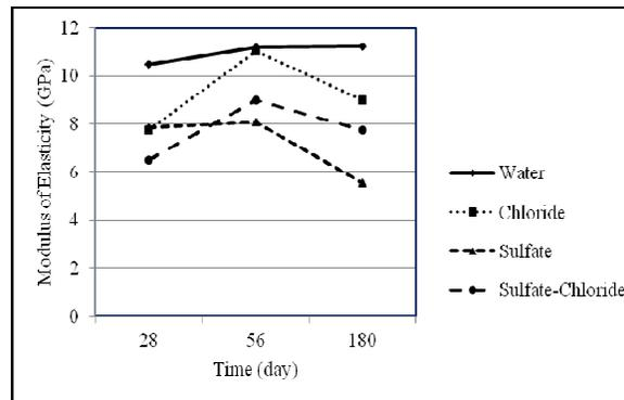
Figure 8: Modulus of elasticity of fired clay brick masonry wall
