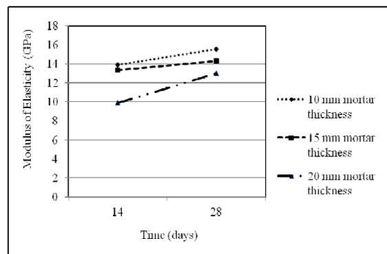
Figure 9: Modulus of elasticity of fired clay brick masonry wall with different thickness of mortar joint
