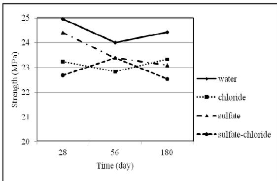
Figure 3: Compressive strength of fired clay brick units
