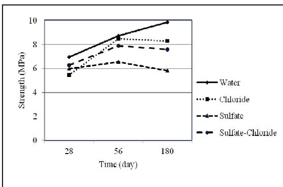
Figure 4: Compressive strength of fired clay brick masonry wall
