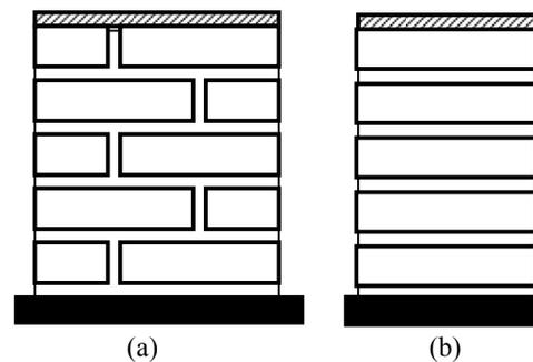
Figure 1: Specimens of (a) masonry wall with 1.5 unit width x 5 unit height (b) masonry prism with 1 unit width x 5 unit height
