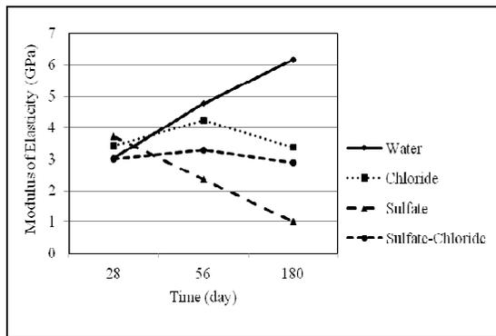
Figure 6: Modulus of elasticity of mortar prism
