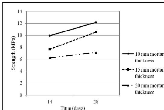
Figure 5: Compressive strength of fired clay brick masonry wall with different mortar thickness
