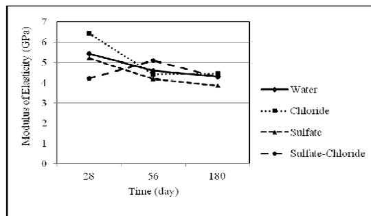
Figure 7: Modulus of elasticity of fired clay brick units
