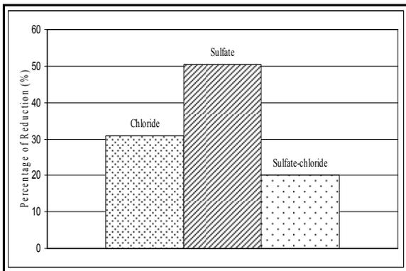
Figure 10: Reduction in modulus of elasticity of fired clay brickwork at the age of 180 days
