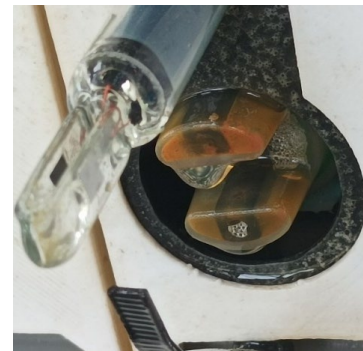
Fig. 9 The water enters the TUR prototype sensor
