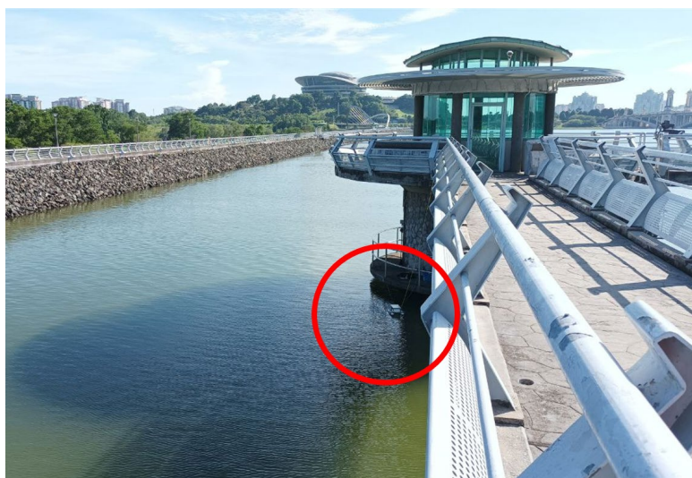
Fig. 10 The shadow of the structure caused insufficient sunlight for solar charging in the evening at Point 1. The red circle shows the location of the IWQM prototype during the deployment period.
