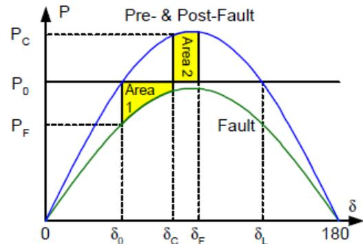
Fig.4 Fast fault clearance and a stable swing
