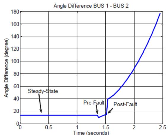
Fig. 9 During unstable condition the angle difference between Bus 1 and Bus 2
