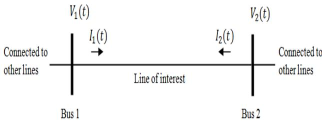
Fig. 6 Transmission line with two-end measurements
