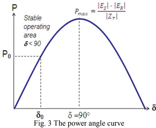
Fig. 3 The power angle curve
