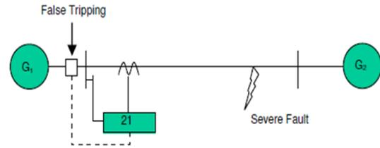
Fig.2 Wrong operation of distance relay due to power swing
