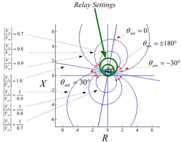
Fig. 7 Measured impedance trajectory in the R-X plane
