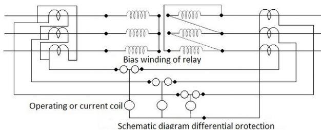
Fig.2 Differential protection scheme
