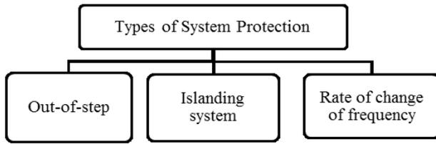
Fig.1 Types of system protection
