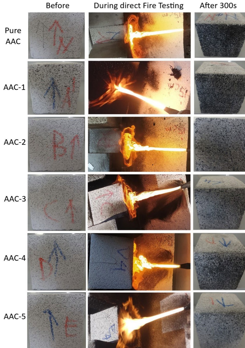
Fig. 3 Pure AAC and AAC-CGW surfaces before, during and after exposure to direct fire testing
