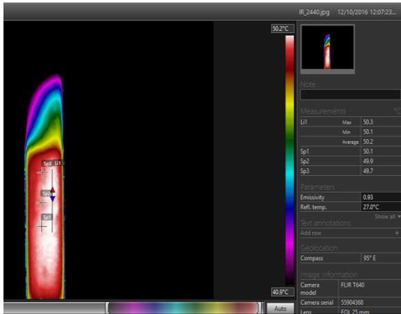
Fig. 4 Thermal image of 60°C hot water
