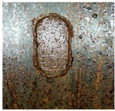
Fig. 9 Artificial wide and shallow pitting in pipe
