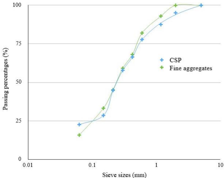
**Fig. 1 - Sieve analysis results for cockle shell powder and fine aggregates**
