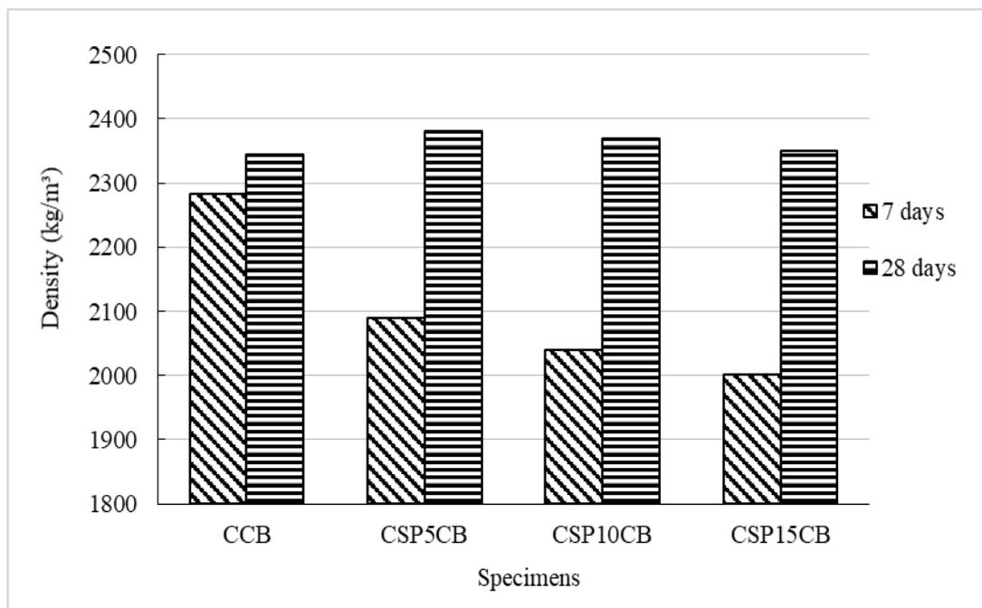
**Fig. 2 - Density of cockle shell cement bricks**
