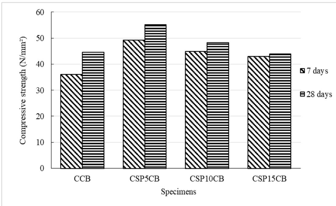
Fig. 4 - Compressive strength of cockle shell cement bricks
