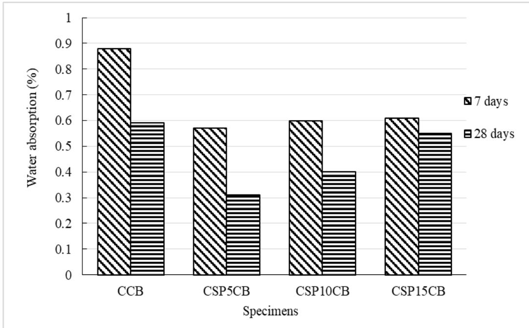
Fig. 3 - Water absorption of cockle shell cement bricks
