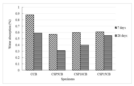
Fig. 3 - Water absorption of cockle shell cement bricks
