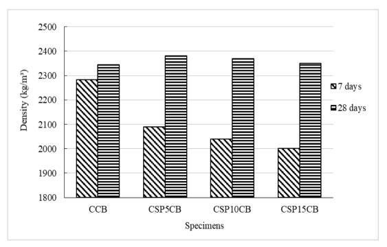
Fig. 2 - Density of cockle shell cement bricks
