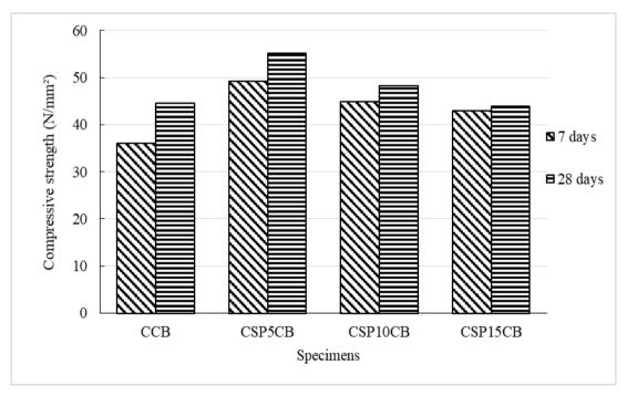
Fig. 4 - Compressive strength of cockle shell cement bricks
