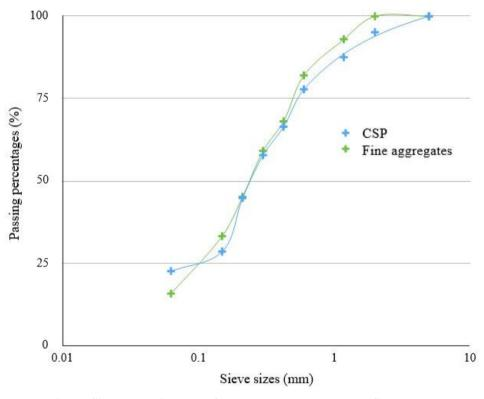
Fig. 1 - Sieve analysis results for cockle shell powder and fine aggregates
