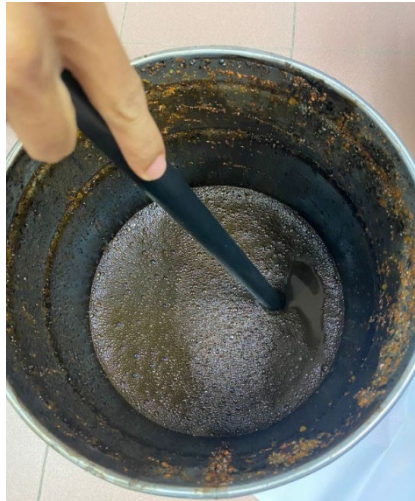
Fig. 5 Mixing and stirring bitumen emulsion before use
