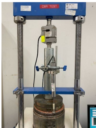
Fig. 8 Performing California Bearing Ratio (CBR) test on soil sample
