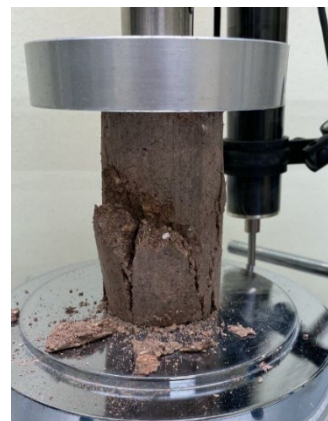
Fig. 9 Conducting the Unconfined Compressive Strength (UCS) test on clayey sand stabilized with 3% cement and 2% bitumen emulsion after a curing period of 7 days
