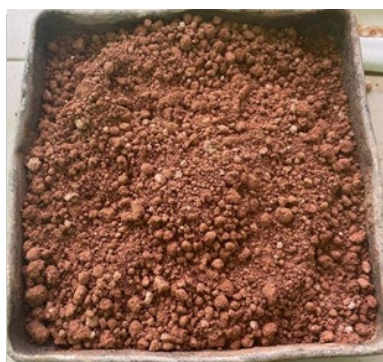
Fig. 3 Clayey sand soil sample
