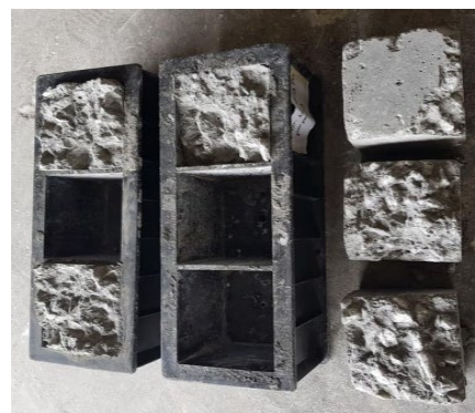
Fig. 4 Unsuccessful concrete un mould for CBC-POM 4
