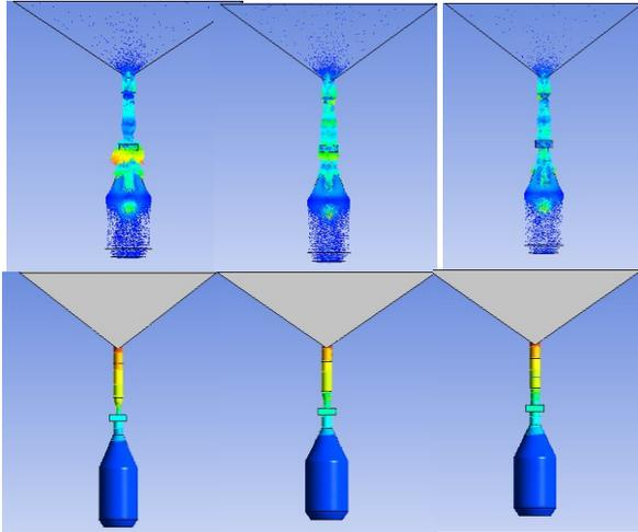
Fig. 5 (a) Velocity vector and (b) pressure contours in a nozzle and bottle at 80°C
