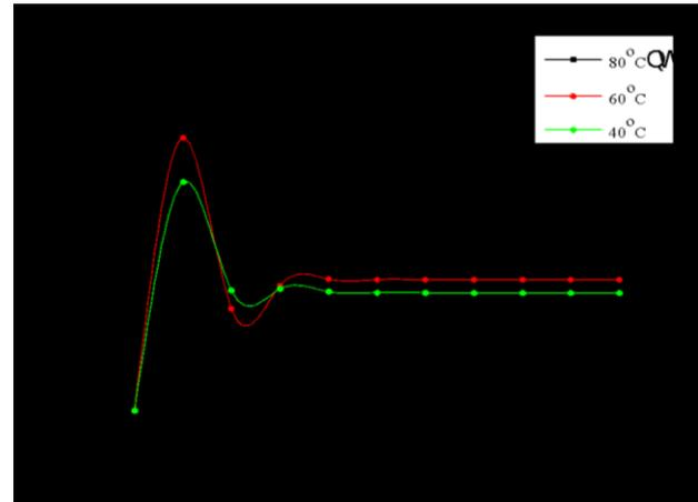
Fig. 4 The flow behavior of chili sauce at different temperatures.
