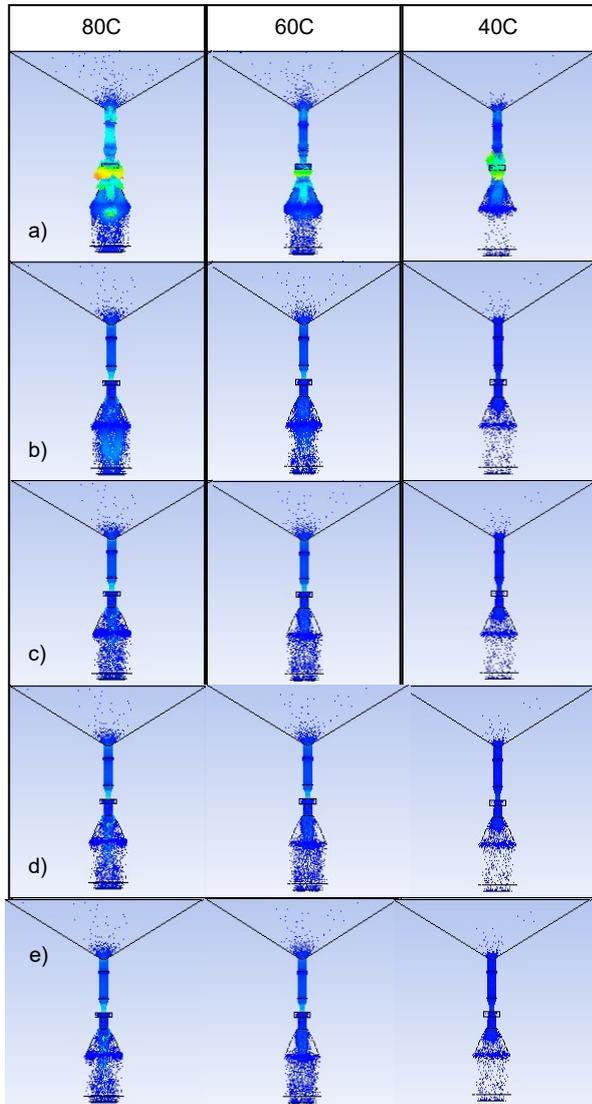
Fig. 3 The flow simulation at 40°C, 60°C and 80°C from 0.15 s to 1.5 second (a) 0.15 sec (b) 0.45 sec (c) 0.75 sec (d) 1.05 sec (e) 1.50 sec
