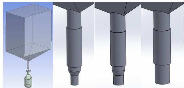
Fig. 1 The dispenser and three different shapes of nozzles
