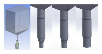
Fig. 1 The dispenser and three different shapes of nozzles
