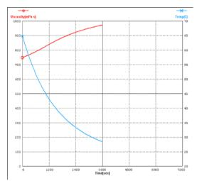
Fig. 6 Viscosity of chili sauce in term of time and temperature
