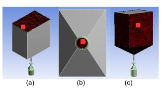
Fig. 2 The boundary conditions (a) inlet (b) outlet (c) wall
