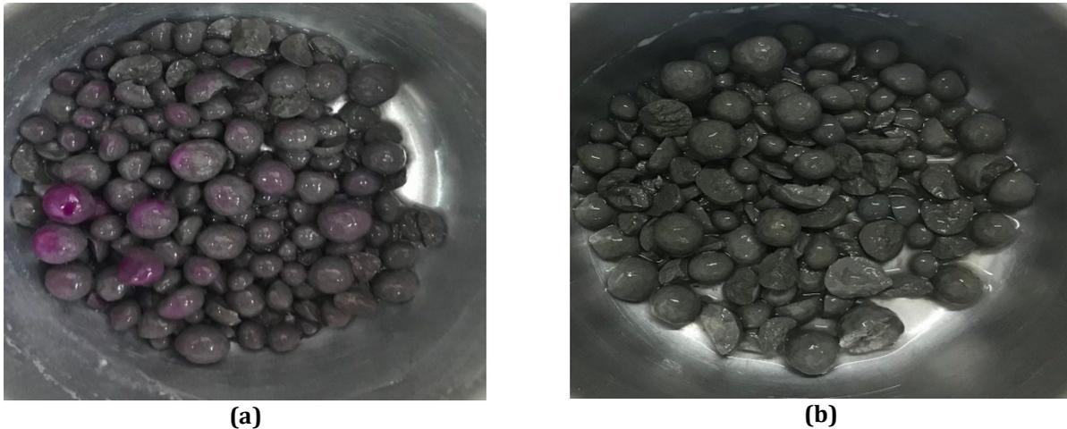
**Fig. 9** Phenolphthalein indication on cement-slag artificial aggregates at different curing regimes (a) CO<sub>2</sub>-water curing (b) CO<sub>2</sub>-air curing
