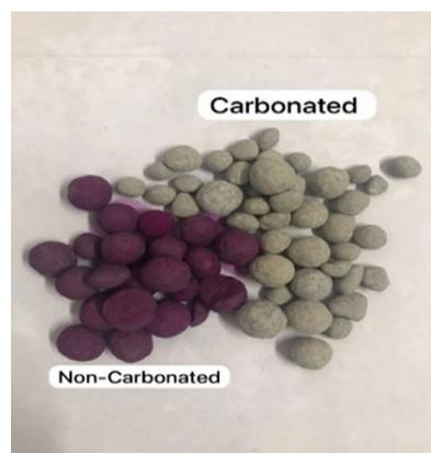
Fig. 5 Visual observation after spraying with phenolphthalein
