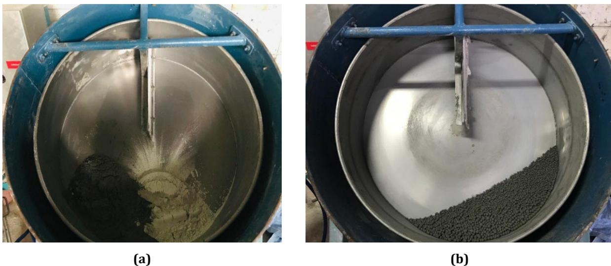
**Fig. 1** Disc granulator (a) Mix of OPC and GGBS; (b) Formation of cement-slag artificial aggregates
