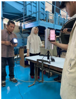
Fig. 16 Testing of the aluminum blade VAWT model in wind tunnel: measuring turbine's rotation, wind speed correspondence, and measuring vibration
