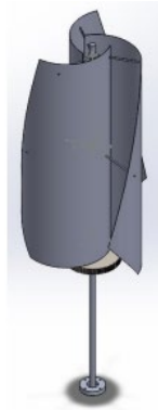
Fig. 8 Design model VAWT according to previous research [14]
