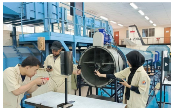
Fig. 17 Testing of the carbon fiber blade VAWT model in wind tunnel
