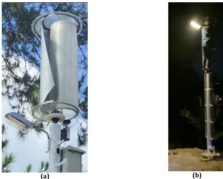
Fig. 7 (a) VAWT current study after assembly; and (b) VAWT test at night
