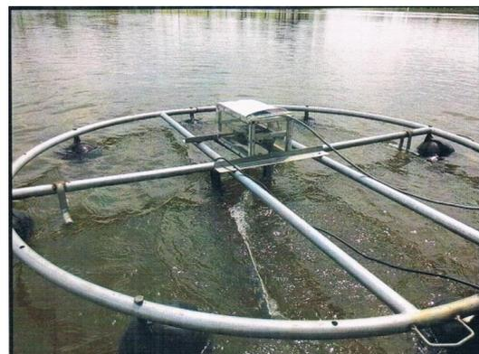
Fig. 1: Flexible Link Aerator
