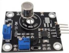
Fig. 6 Nitrogen dioxide sensor
