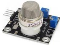
Fig. 5 Sulphur dioxide sensor
