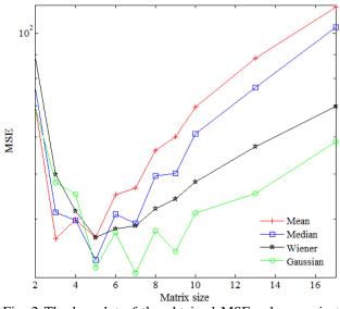
Fig. 2 The log plot of the obtained MSE values against different matrix sizes for the employed filters.
