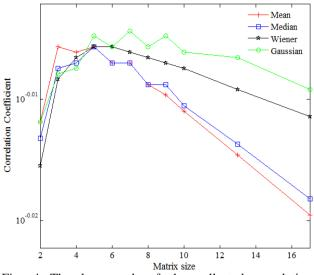
Fig. 4 The log graph of the collected correlation coefficients for different employed filters versus various matrix sizes.
