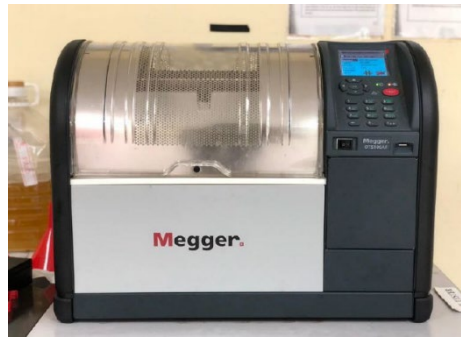
Fig. 1 Megger OTS100AF oil breakdown tester
