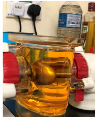
Fig. 2 400 ml oil test cup
