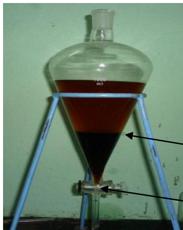
Fig. 3 Separation of biodiesel & glycerine
