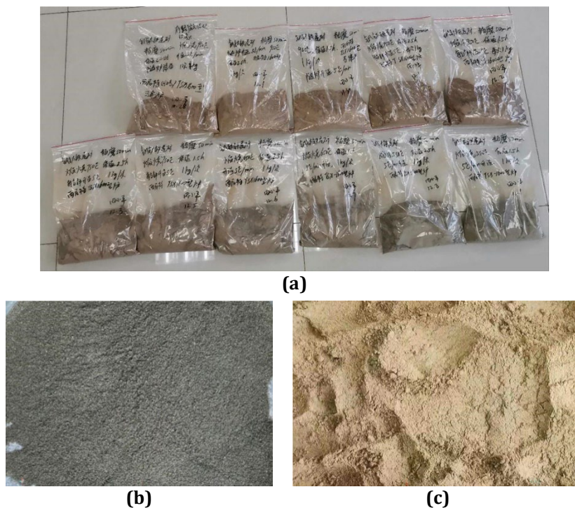
Fig. 3 VTIoT specimens colour comparison: (a) The VTIoT at different calcination temperatures; (b) The uncalcined VTIoT; and (c) The VTIoT after calcination at 950°C
