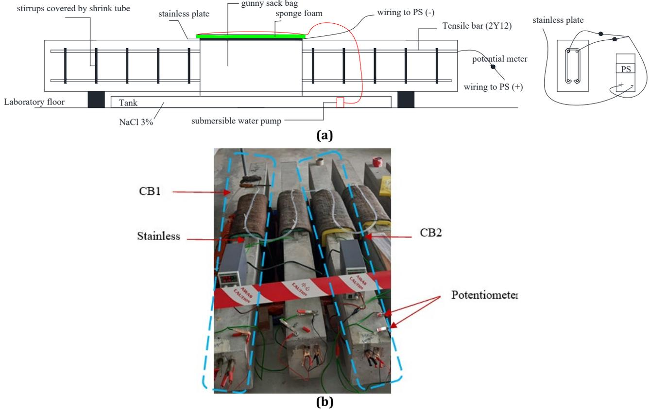
Fig. 2 Accelerated corrosion (a) detail setting up; and (b) application of accelerated corrosion to test objects
