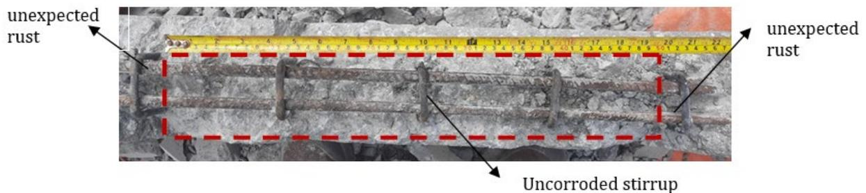
Fig. 11 Rust on tensile reinforcement
