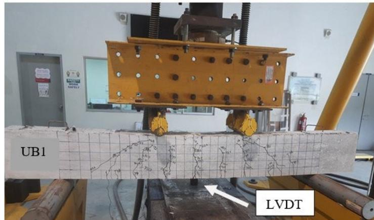
Fig. 5 Static loading test system
