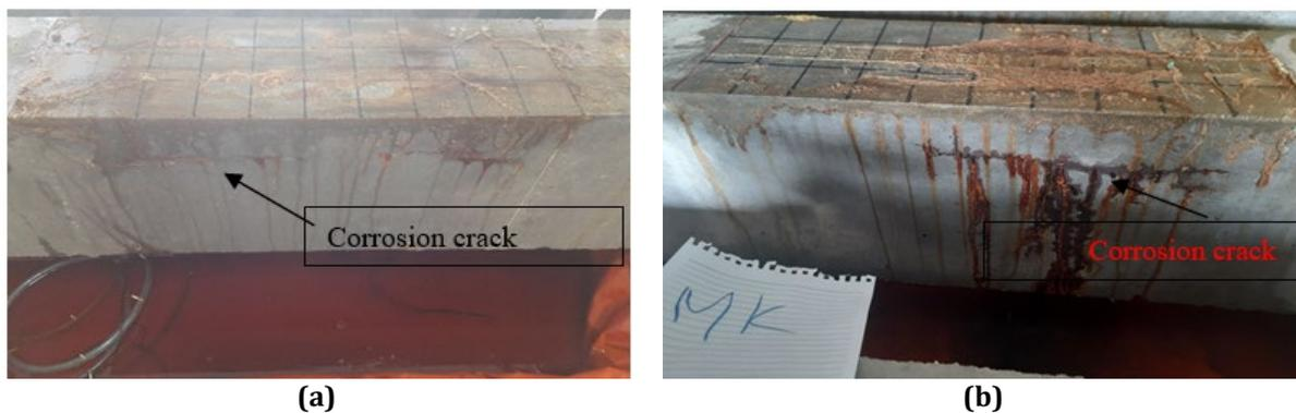
Fig. 7 Corrosion crack (a) CB1 horizontal crack; (b) CB2 horizontal crack
