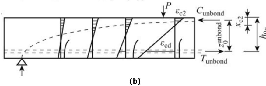
Fig. 10 Equilibrium of forces and compatibility of deformations (a) bonded beam; (b) unbonded beam
