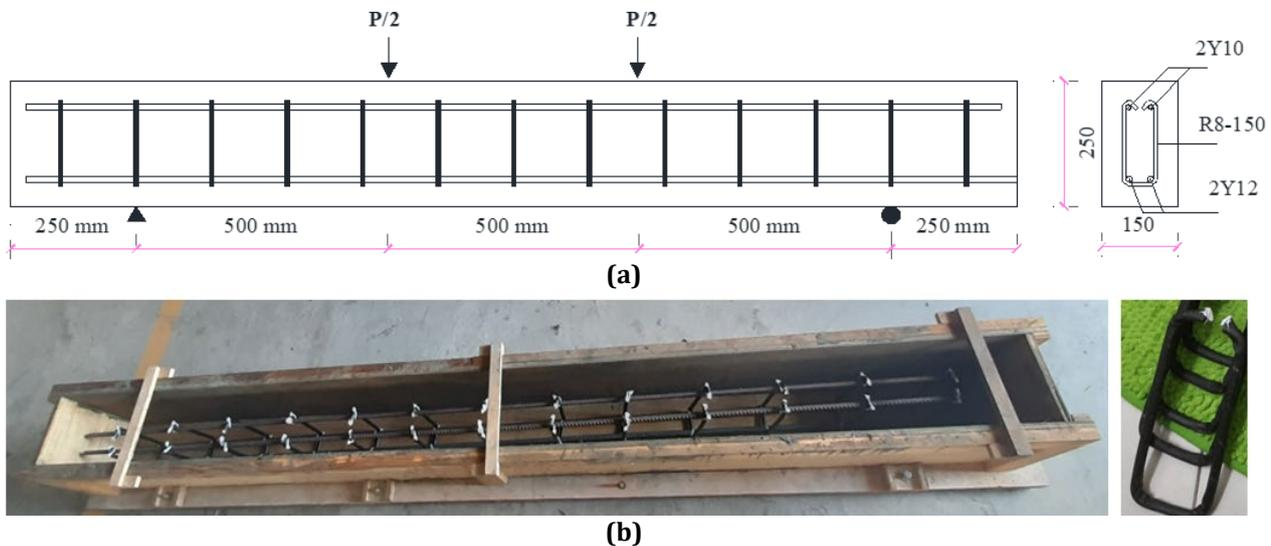
**Fig. 1** Beam (a) reinforcement detail; (b) installation of shrink tube on the stirrup
