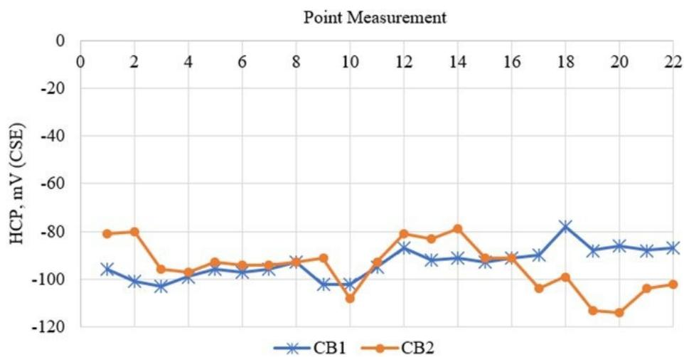
Fig. 6 Half-cell potential data
