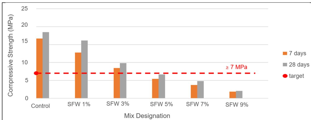
Fig. 4 Compressive strength at 7 and 28 days
