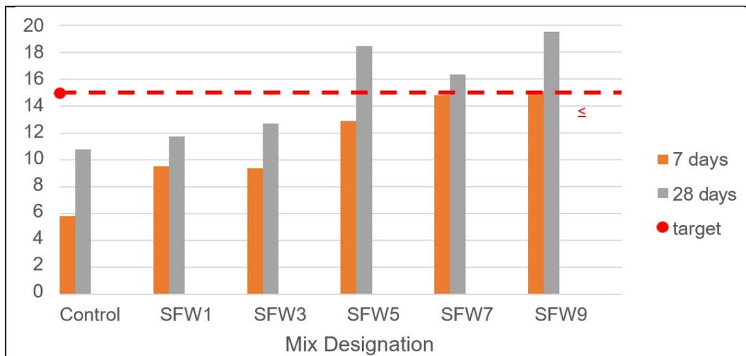
Fig. 5 Water absorption at 7 and 28 days
