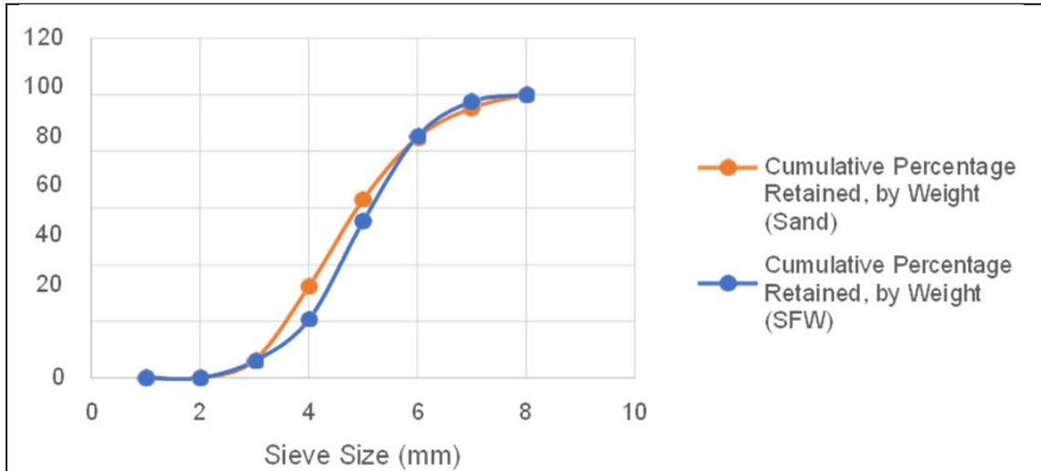
Fig. 2 Grading curve of sand and SFW
