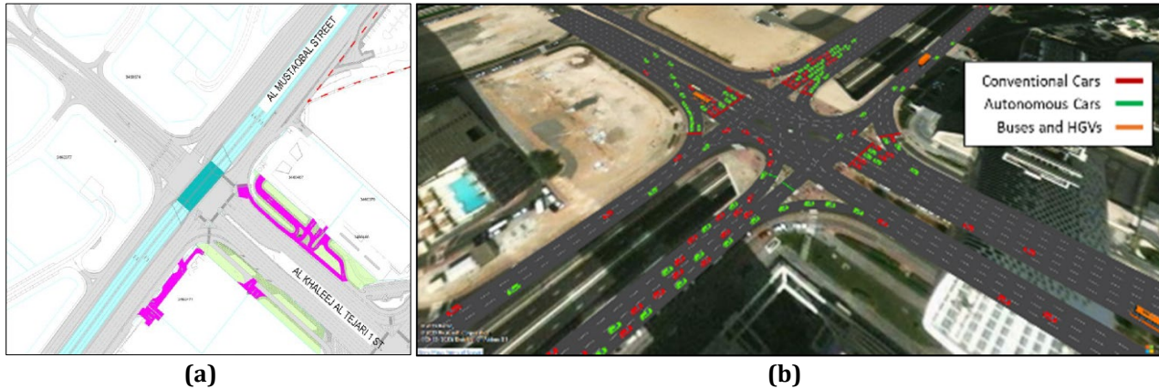
Fig. 4 The considered study site; (a) plan layout of the site geometry; (b) simulation run on base model in VISSIM
