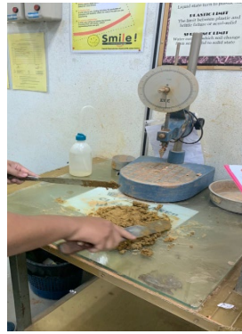
Fig. 6 Atterberg limit test including Liquid limit (LL) and Plastic limit (PL)
