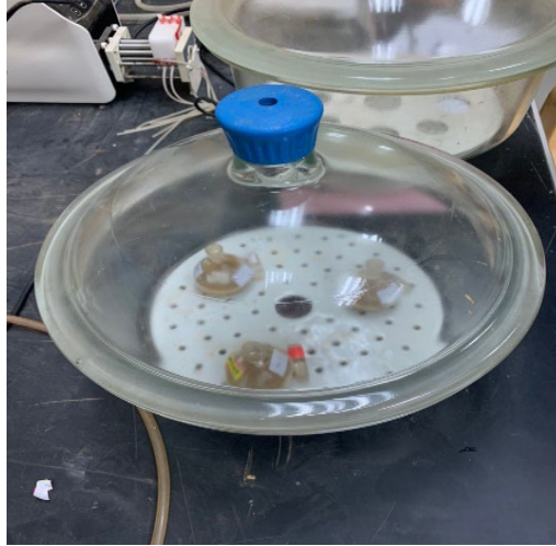
Fig. 4 Pycnometer method for determining specific gravity
