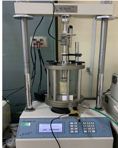
Fig. 8 Consolidated Isotropic undrained (CIU) testing with model VJ Tech
