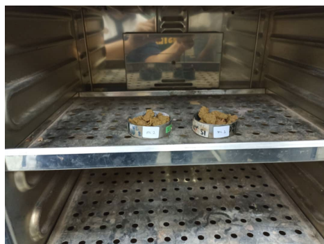
Fig. 3 Oven drying process for determining moisture content
